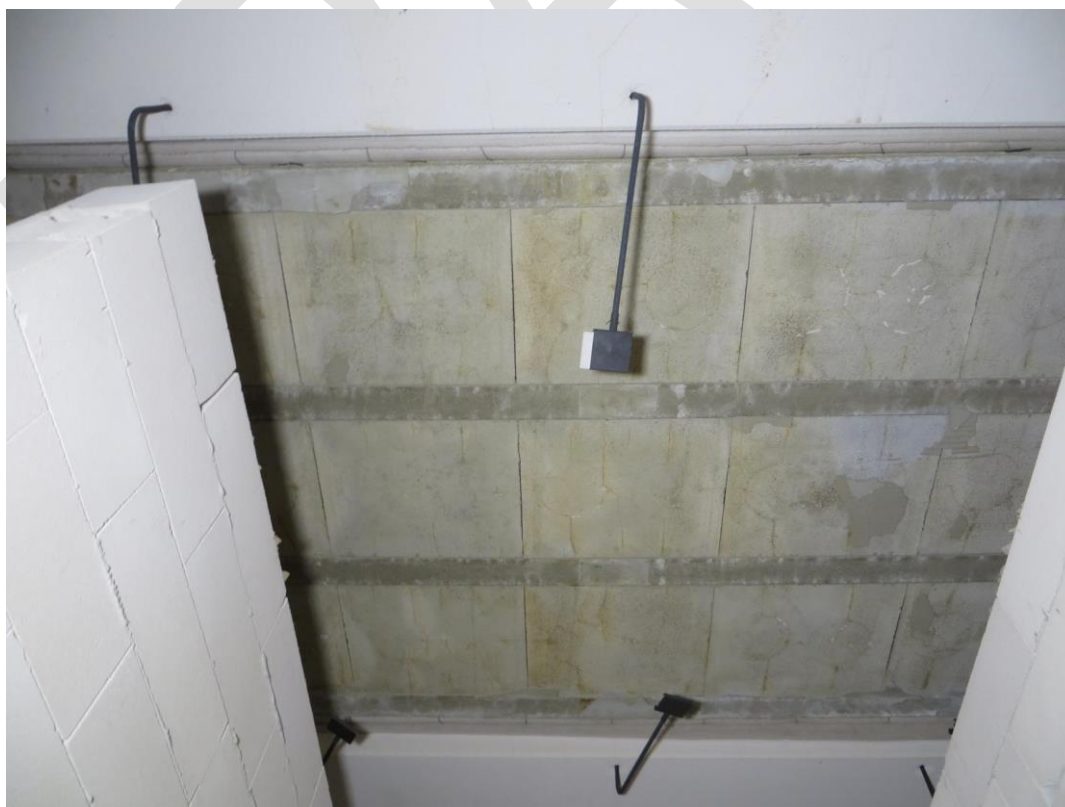
Photo No. 046997d-162: exposed face at the end of the test
