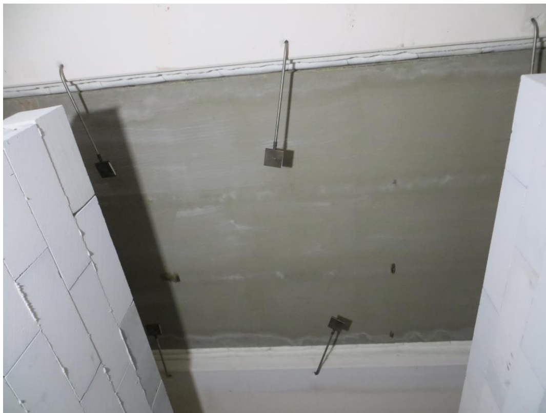
Photo No. 046997d-028: exposed face before the commencement of the test
