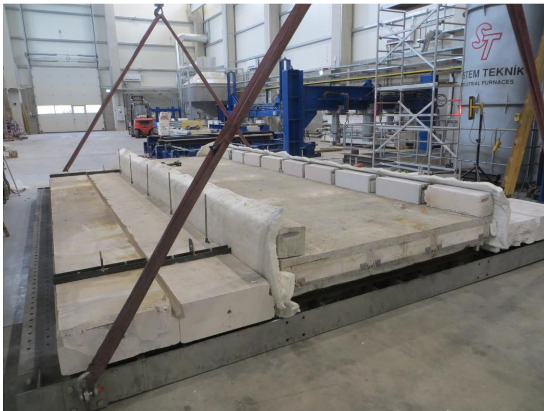
Photo No. 046997d-019: test specimen placed on the test frame and slabs placed at the longer edges
