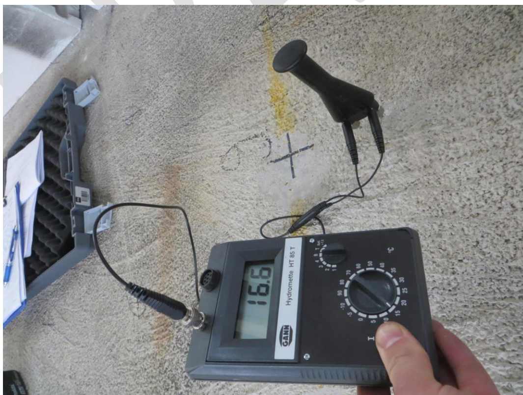
Photo No. 046997d-025: measuring of moisture content in the test specimen
