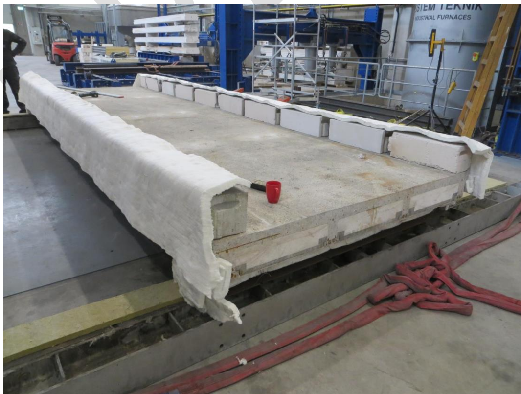
Photo No. 046997d-002: test specimen laid on the supporting construction
